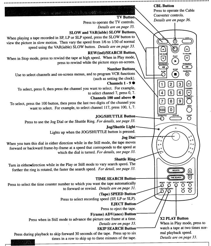
Shaded boxes indicate TV control and cable converter box control buttons. They may or may not operate your TV or cable converter box. See pages 35 and 36 for details.
